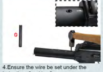
4. Ensure the wire be set under the hole, then fixed by G.
