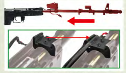
4. Assemble Red Area to Receiver and put the Wire Assembly of Gear Box into groove. (as picture of green frame)
