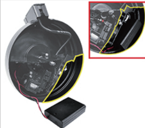
4.將電池盒置入黃框處。 Place the battery holder in the yellow circle mark.
